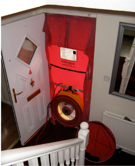
Air Tignness Testing Westerdale Place
